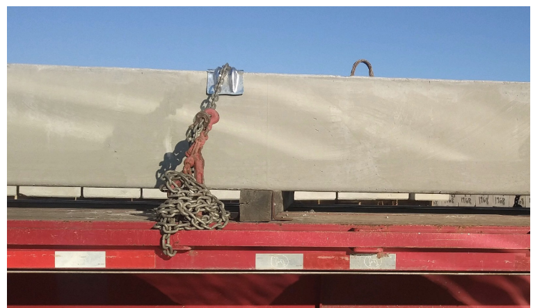
Correct—chain guards are firmly in place
