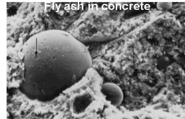
Electron Micrograph Fly Ash in Fresh Concrete
