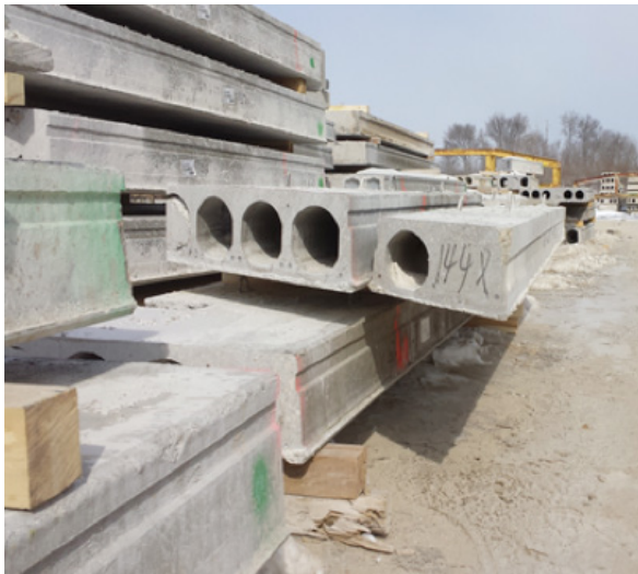
Uneven stacking; dunnage not aligned
