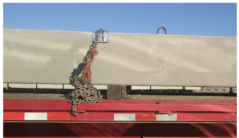
Correct—chain guards are firmly in place
