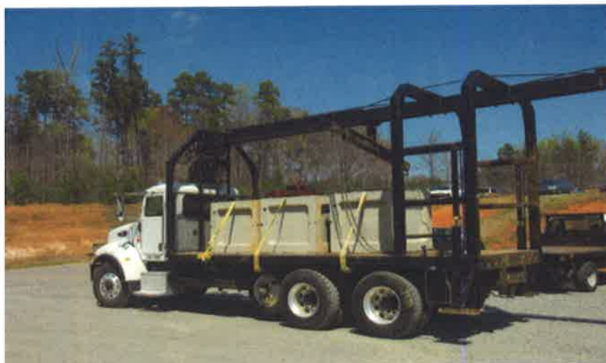
Photo 1: Septic Tank Delivery Rig
