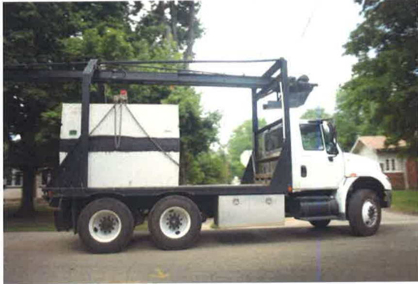
Photo 2: Septic Tank Delivery Rig
