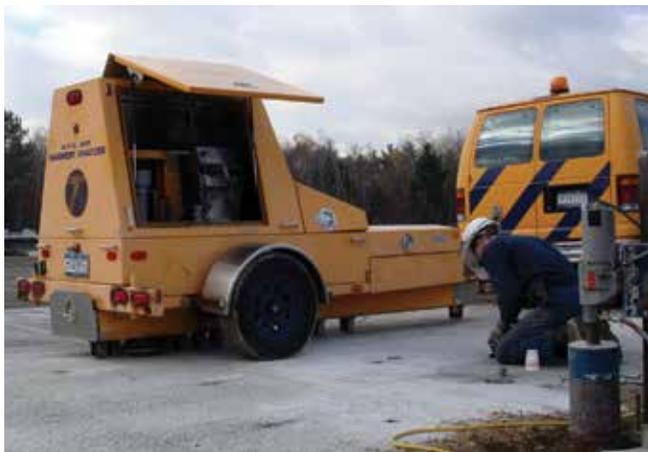
**Figure 13: Falling weight deflectometer testing device**
