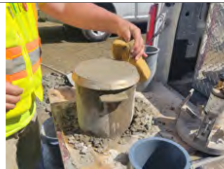
Cleaning edge of bucket before air test.
