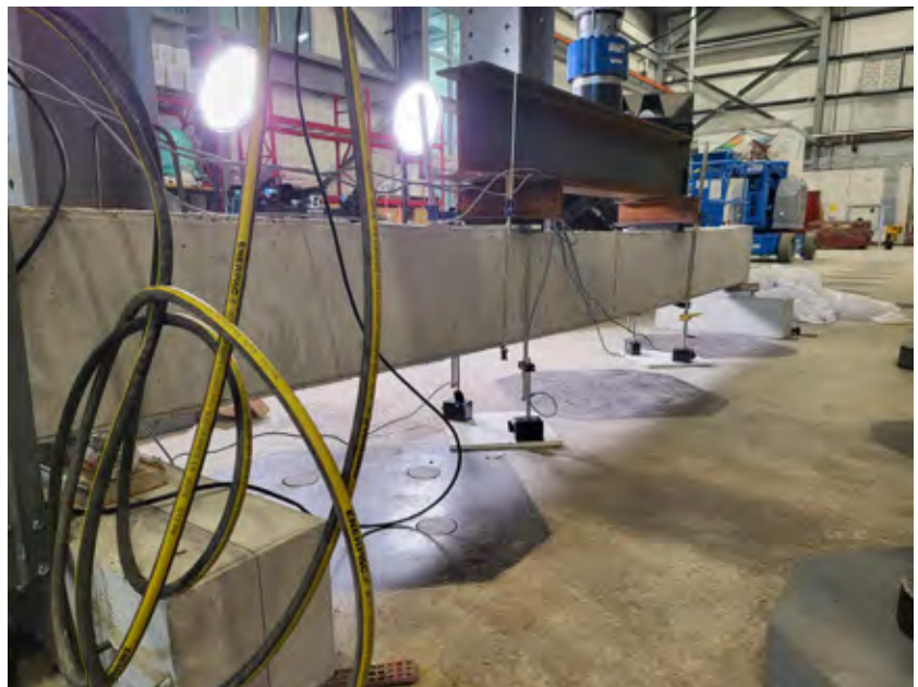
A precast beam made with BCSA (Belitic calcium sulfoaluminate) undergoing flexural testing at Oklahoma University.
