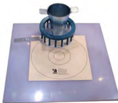
J-Ring Test Set, including a slump cone, straightedge, heavy-duty steel J-Ring and a large, rigid plastic base plate with centering ring decal on which to perform the test.
