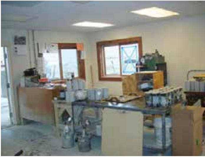
Figure 10-3. Entrained air meter and compression testing equipment in a precast plant testing lab.
