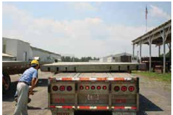
Figure 7-7. Warped-plane panel with a 4-inch delta (warp) on a truck.
