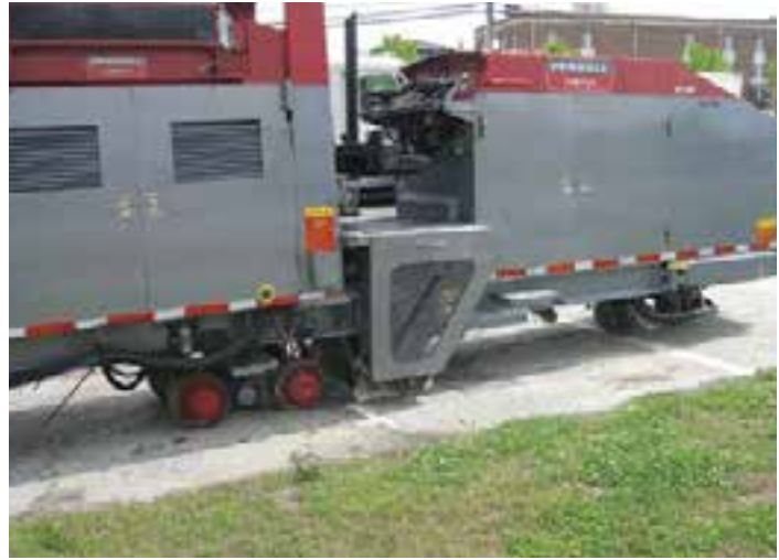
Figure 11-22. Typical diamond grinding profiler with grinding head near the center of the photo. The bogie wheels on the left control the cross-slope of the head while the dual in-line center wheels on the right establish the longitudinal profile of the grinding machine.
