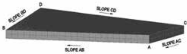
Figure 2-21. Schematic of non-planar pavement surface where opposite sides always have different slopes.
