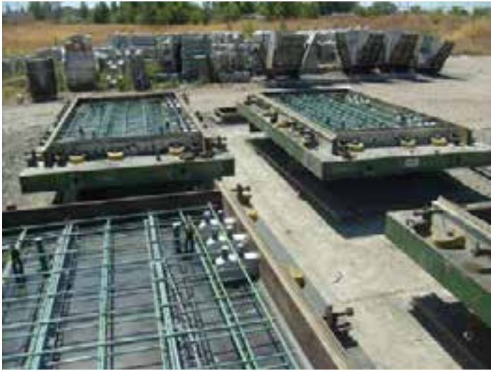
Figure 7-3. Individual, adjustable-width forms.
