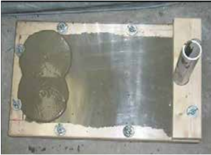
Figure 9-13. A flow chamber equipped with a Plexiglass bottom to allow observation of simulated grout flow under a panel as it fills a void that varies from 0 to 1/4 inch deep.
