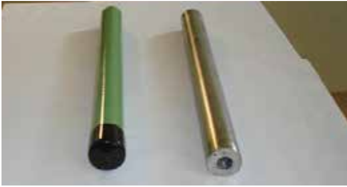
Figure 13-6 A flanged nut is welded inside both ends of a tubular stainless steel Super-Dowel, shown at right. An epoxy-coated tubular carbon steel dowel, capped and ready for installation, is pictured on the left.
