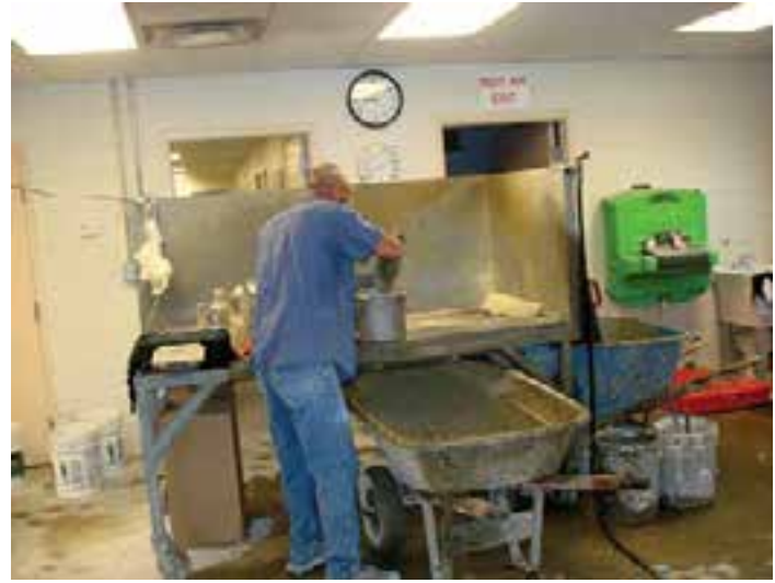
Figure 10-4. An American Concrete Institute-certified concrete technician measures air content.
