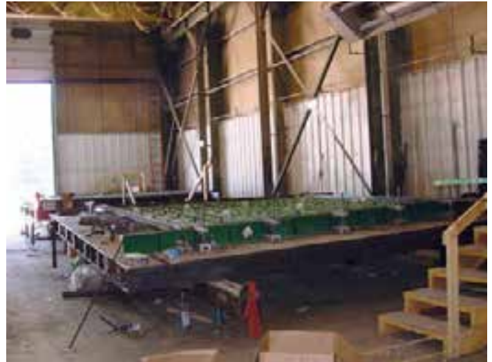
Figure 7-6. This photo shows one corner of the bed, "D," lowered by the specified "Delta" distance below the plane defined by the other three corners, which are supported in a level position.
