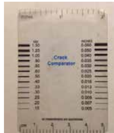
Figure 11-8. A simple crack comparator used to estimate crack widths in inches or millimeters.
