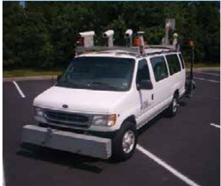
Figure 12-2. This digital survey vehicle gathers data while traveling at or near highway speeds.
