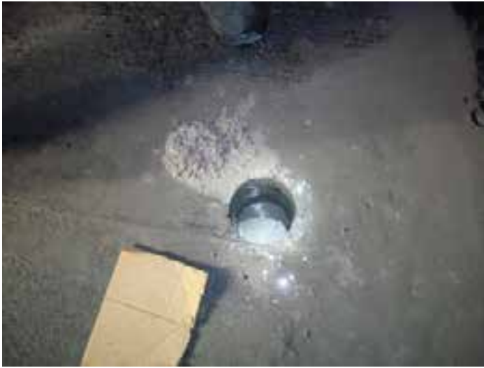
Figure 2-14. Water standing in a core hole several minutes after retrieval, indicating poor drainage of underlying layers.
