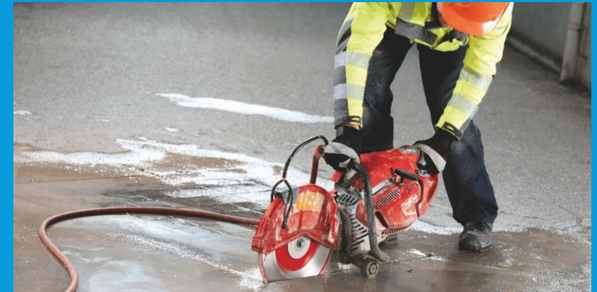
Saw with Vacuum attachment
