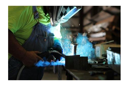
Different welding processes can expose employees to more specific hazards in the fumes. The PEL for nonspecific welding fumes is 5 mg/m3 (milligram per cubic meter).
