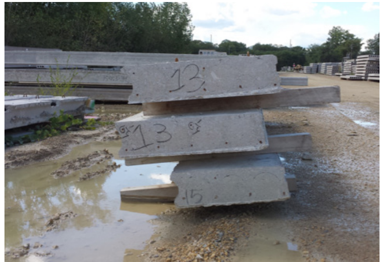
Misaligned stacking, tilted stack, and soft ground
