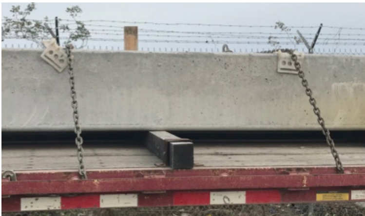
Incorrect—chain guard is loose
