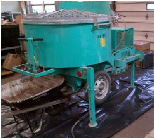
Figure 1 (top left) – High shear mixer; Figure 2 (left) – Small (14-50 bags mixer); Figure 3 (above) – UHPC batching facility. (Photos courtesy of Lafarge)
