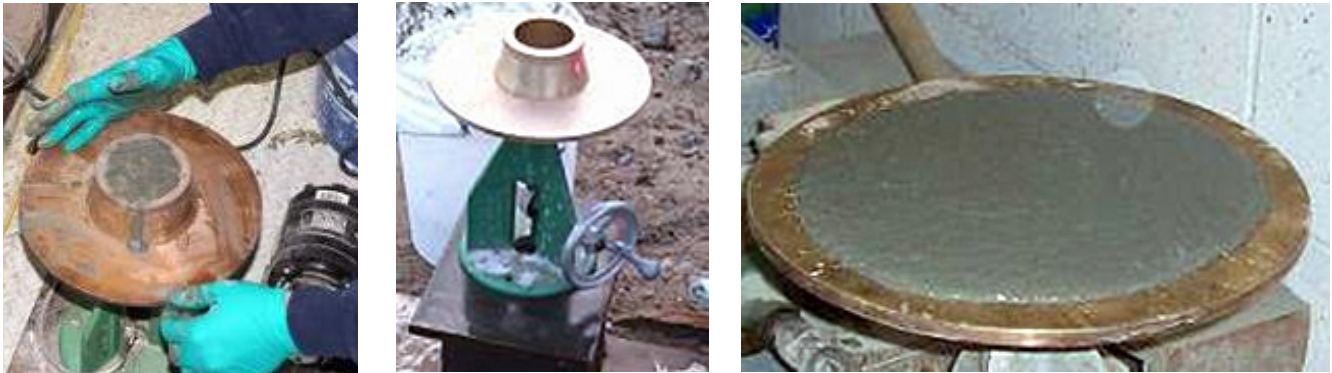
Figure 8 – The plastic flow of each batch is determined in accordance with ASTM C230.
