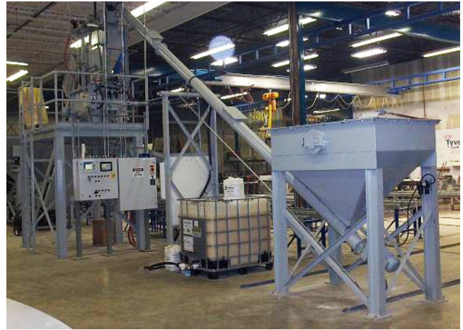
Figure 1 (top left) – High shear mixer; Figure 2 (left) – Small (14-50 bags mixer); Figure 3 (above) – UHPC batching facility. (Photos courtesy of Lafarge)
