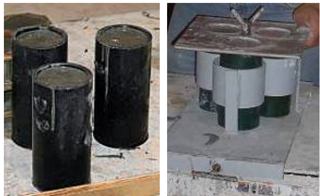
Figures 9, 10 – UHPC compressive strength cylinders (left); vibration of UHPC compressive strength cylinders (right).
