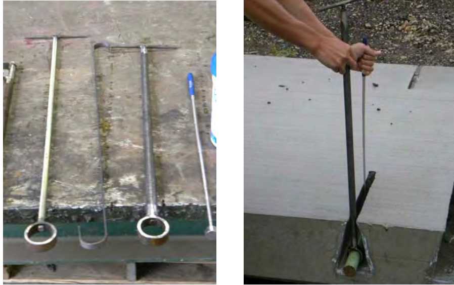
Figure 14.10. Tools to facilitate sliding the dowel bars in the slots and holding the bars in place.
