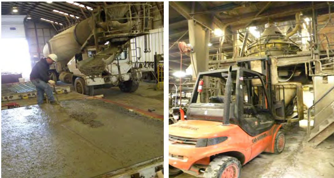
Figure 9.6. Concrete delivery options (transit mixer and bucket).
