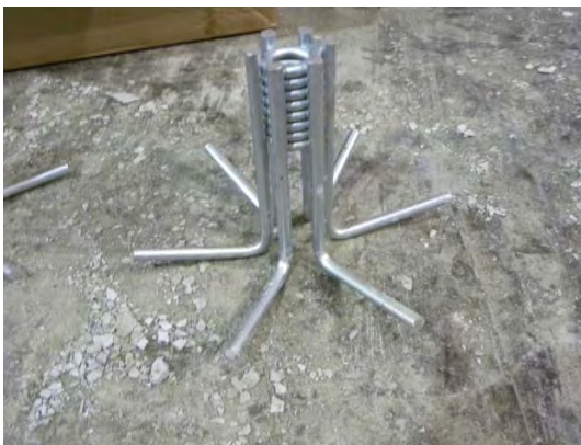
Figure 4.3. Lifting anchors. (By permission of FMC)
