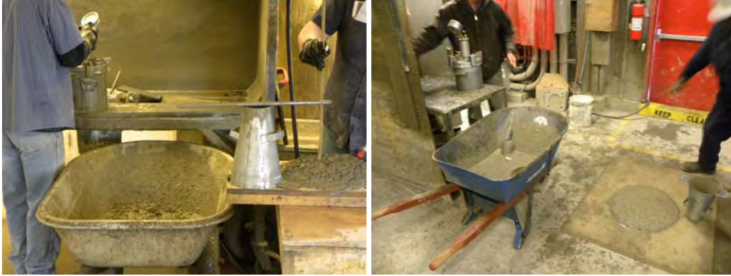
Figure 9.10. Views of concrete quality testing at precast plants.
