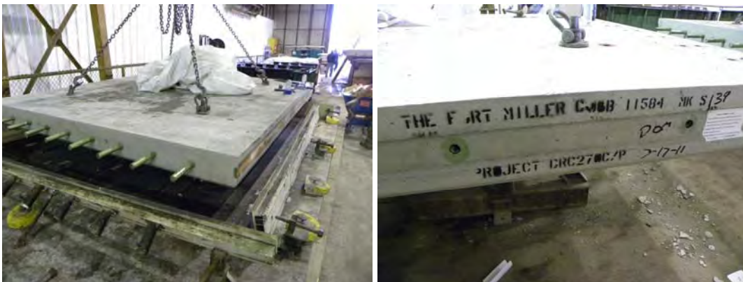
Figure 9.9. Stripped panel being moved to another location.
