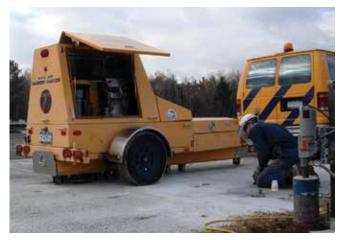
Figure 13: Falling weight deflectometer testing device
