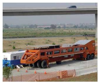
Figure 14: Heavy vehicle simulator testing device
