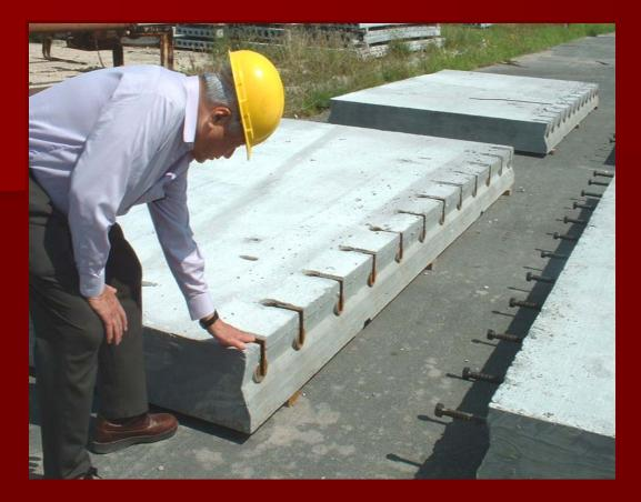
KWIK JOINT couplers are cast into the KWIK SLABS at the precast yard.
