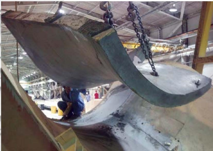
with varying horizontal striations. The panel design incorporates both convex and concave horizontal striations. “The random combinations lend striking shadows, and the striations give way to smooth concrete surfaces on higher levels of the building,” according to the case study.
