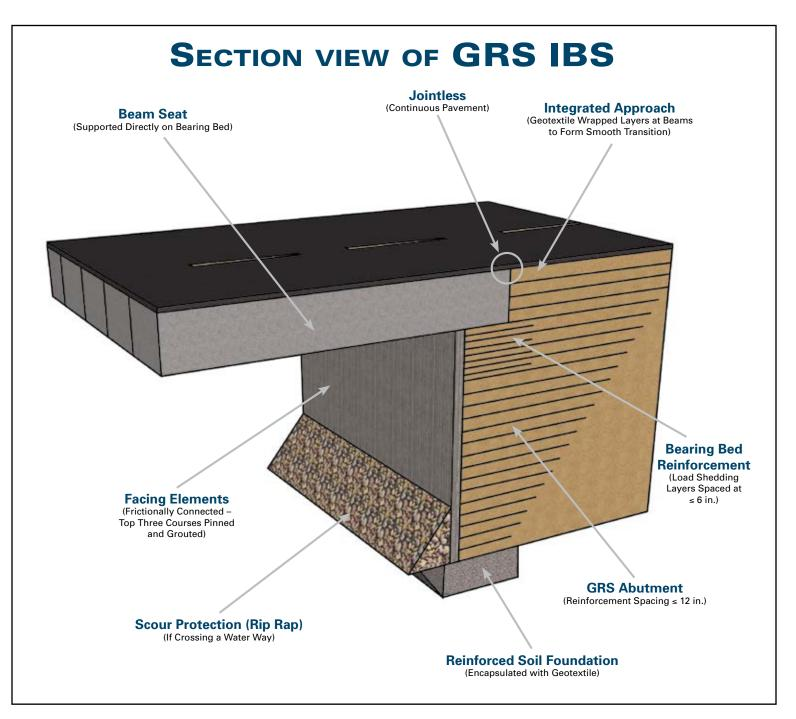
constructed faster at lower costs and with improved worker safety and structural durability.
