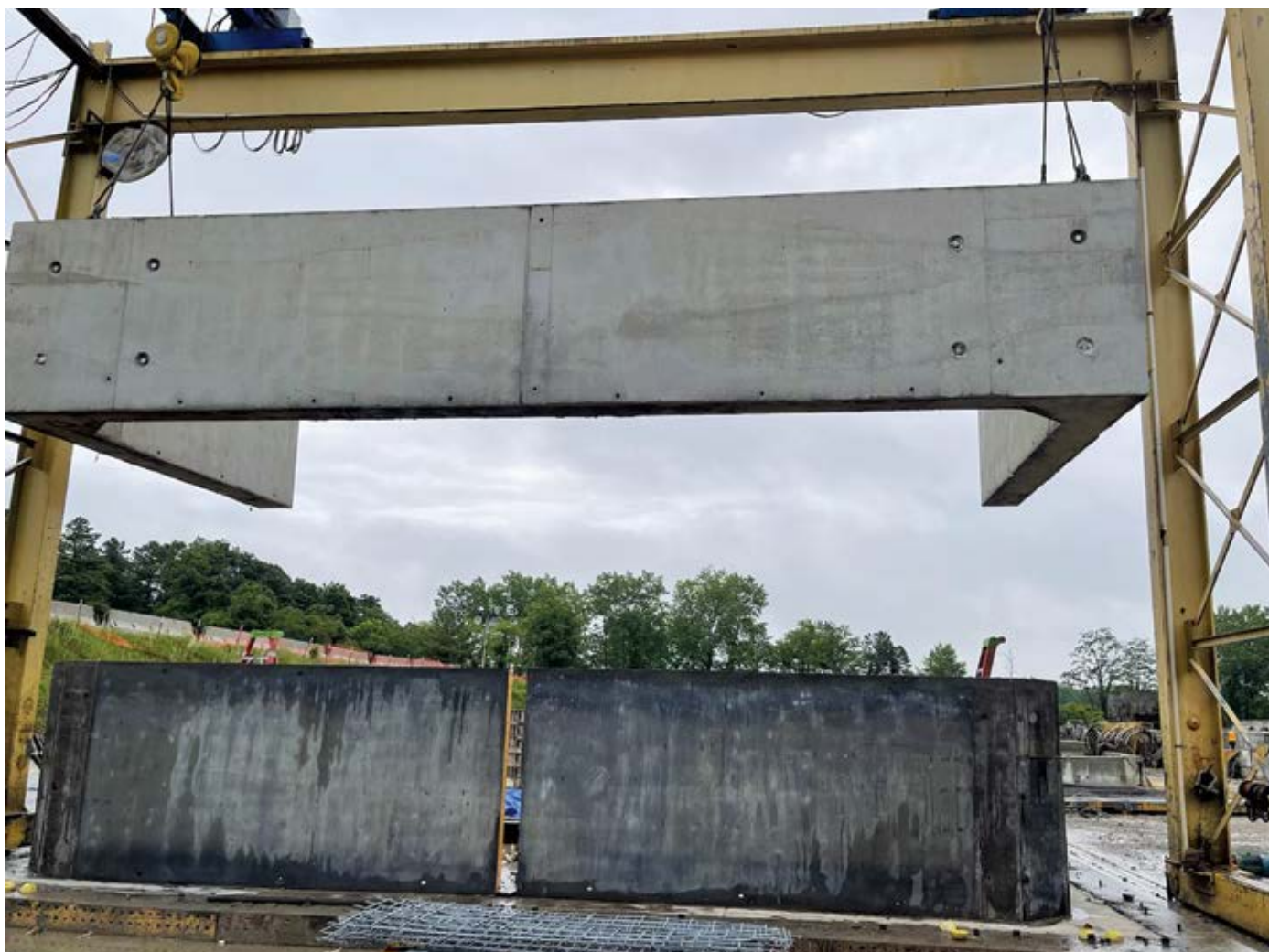
A culvert section is removed from its formwork and lifted by a crane at Garden State. Production for this project is taking place outdoors due to the size and weight of the culvert sections.
