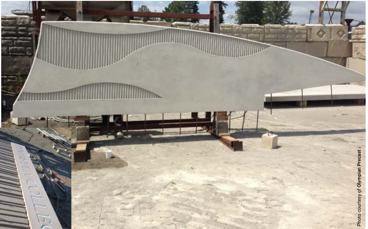
(Above) Olympian Precast produced ribbed precast concrete signs for a local community's multiphase gateway project. (Left) The company also manufactured a monument sign for Peninsula College that included an integral pigment and two different finishes.
