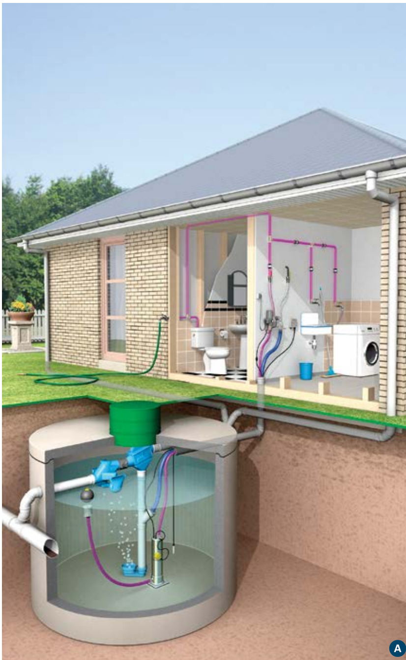
RH20's underground precast rainwater harvesting systems helped reduce overall water discharge flows by 60% for a neighborhood in Newmarket, Ontario.
