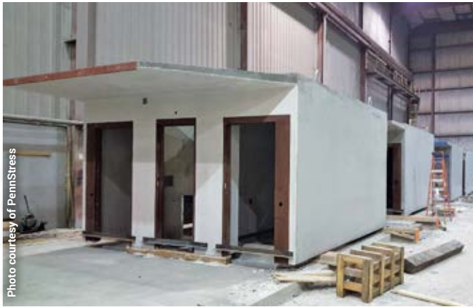
PennStress manufactured 128 precast concrete jail cells. By using precast concrete and modular construction, crews were able to quickly build the correctional facility.
