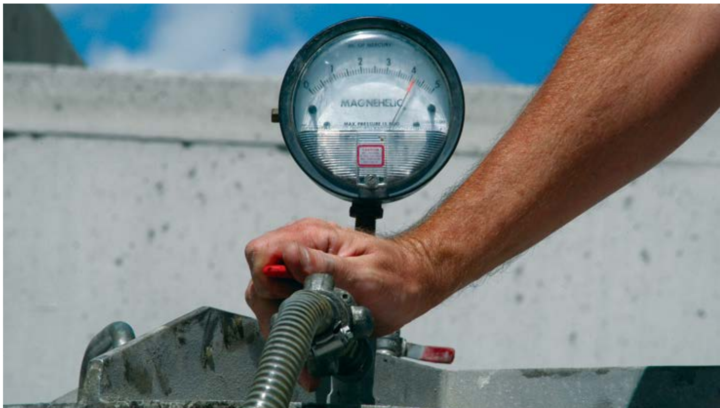
A tank is considered to have passed the vacuum test if the pressure is held at 4 inches Hg for a duration of 5 minutes.
