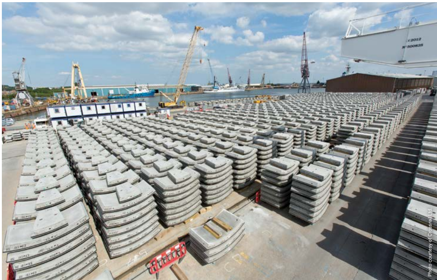
Rows of precast concrete segments await transport at Chatham Dockyard.
