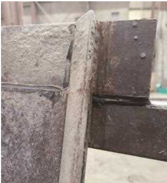
Figure 2: Chamfer at precast formwork corner
