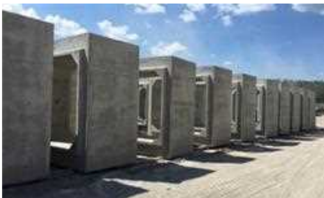
Box culverts are staged to ship from Mack Industries.
