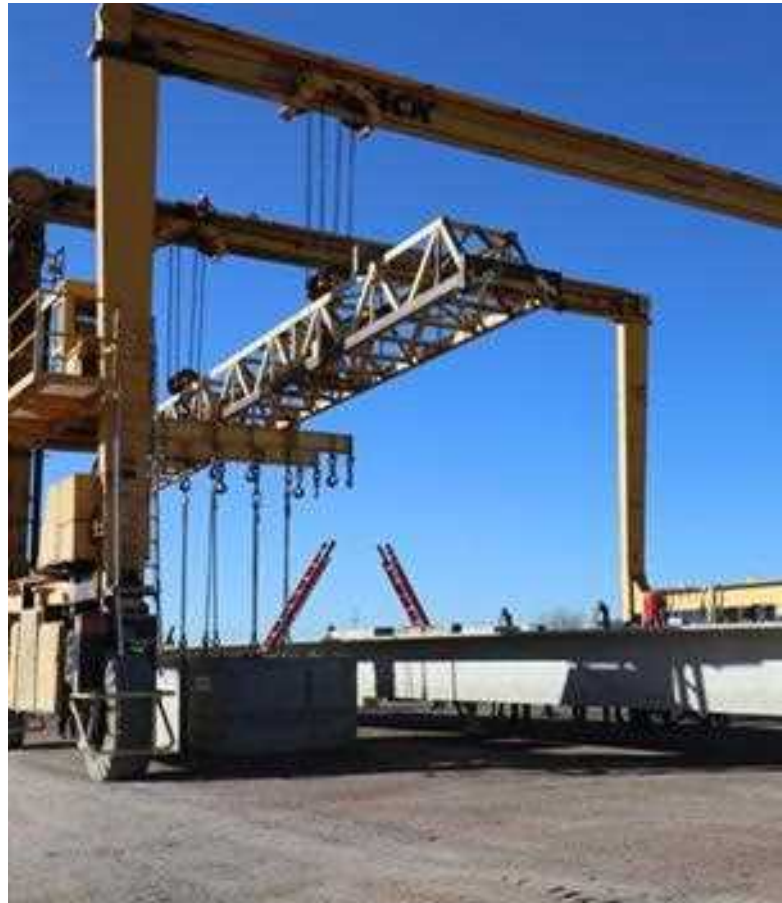
Stresscon conducts a double-tee load test for visitors to observe during the plant tours.
