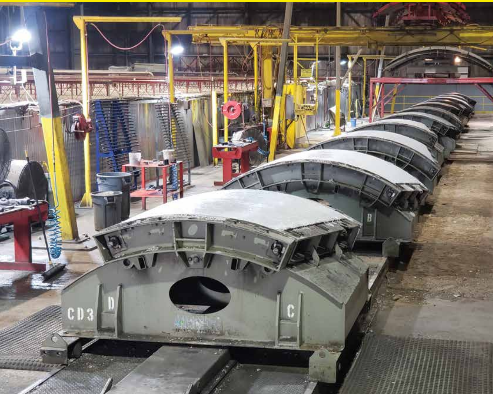
CSI Tunnel Systems will manufacture more than 20,000 precast concrete segments to line the Lower Olentangy Tunnel in Columbus, Ohio.
