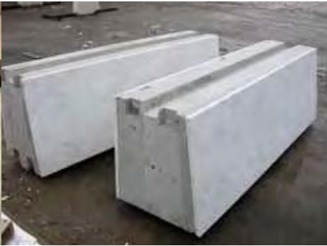
MARBLE-CLAD PRECAST SECTIONS FOR THE FLIGHT PATH WALL, SHOWN IN THE ROYAL STONE PRODUCTION PLANT. Photo by Bruce Felix, AKJV
