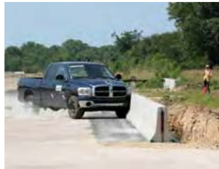
EASI-SET'S J-J HOOKS BARRIERS DURING CRASH TESTS
