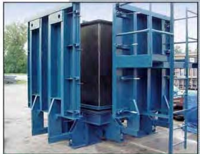
CATCH BASIN WITH ROLL BACK JACKETS
