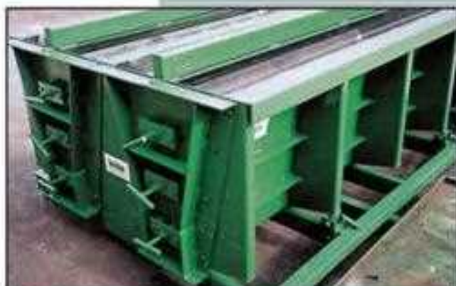
DUAL-CAVITY MEDIAN BARRIER FORM
