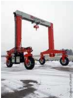
Shuttlelift's new SB 120 single-beam, single-hook, rubber-tired mobile gantry crane
