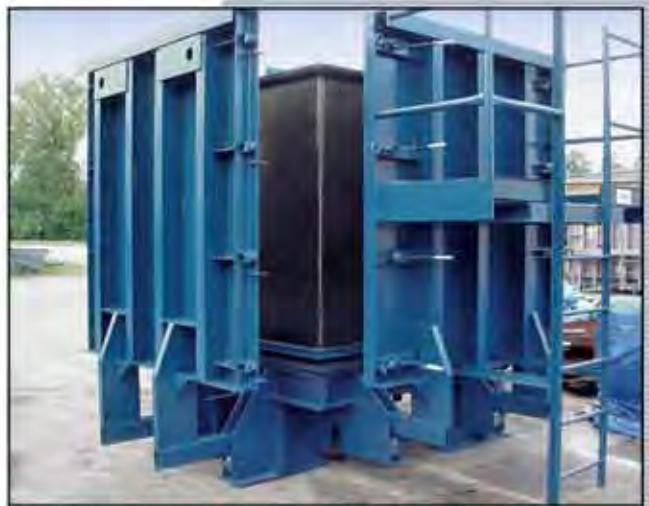
CATCH BASIN WITH ROLL BACK JACKETS
