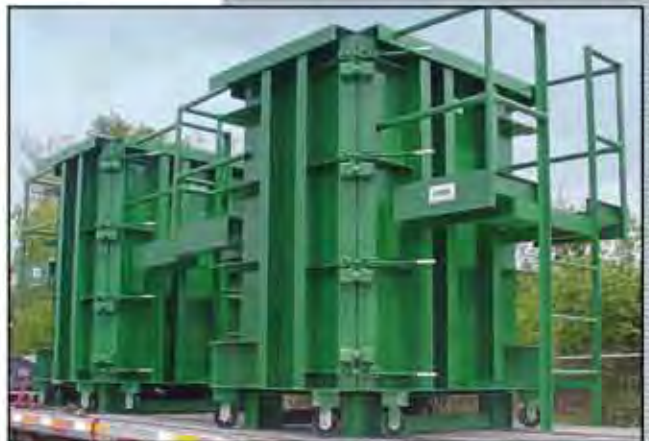
CATCH BASIN FORM WITH FLYAWAY JACKETS
