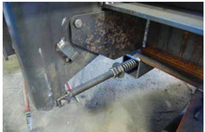
CHECK VIBRATOR MOUNTS, SPRINGS, HINGES AND MOVING PARTS FOR PROPER OPERATION AND RANGE OF MOTION.
