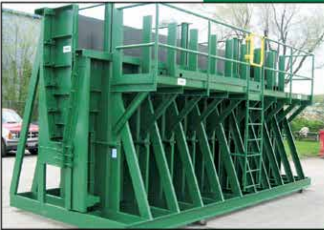
ASYMMETRICAL MEDIAN BARRIER FORM
