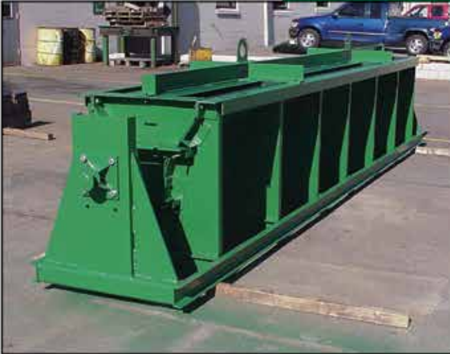
SINGLE FACE MEDIAN BARRIER
