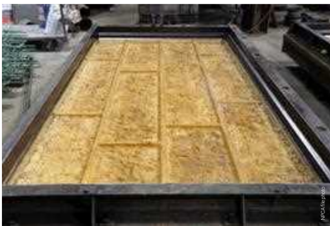
Polyurethane formliners give precasters endless design options.
