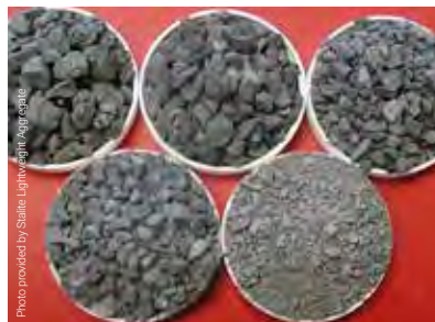
Aggregate porosity and angularity may create mixing challenges compared with conventional aggregate batching.
