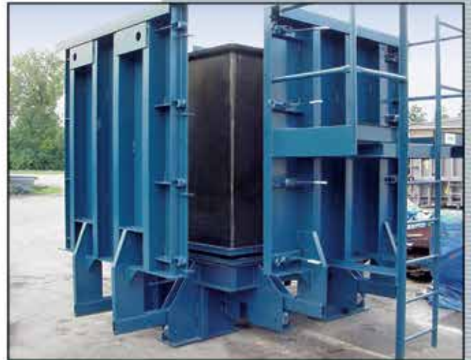
CATCH BASIN WITH ROLL BACK JACKETS
