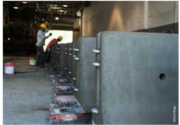
A dry-cast product can be immediately stripped from its form and can stand on its own to complete the curing process.
