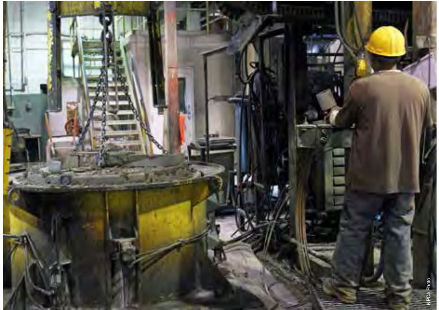
A heavy-duty form is needed to manufacture dry-cast precast concrete products.
