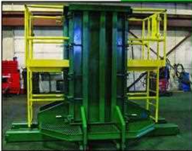
CATCH BASIN WITH ROLL BACK JACKETS
