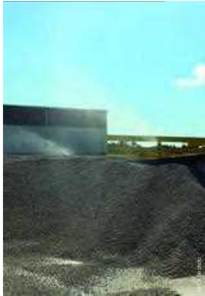
Wetting or watering aggregate stockpiles with a sprinkler system can help cool the aggregates.
