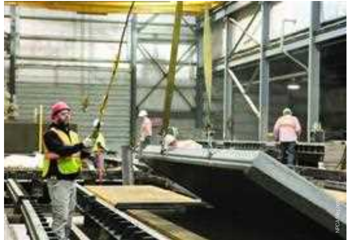
Many crane operators can operate the crane on the production floor without the need for a specific signal person by using a remote control.
