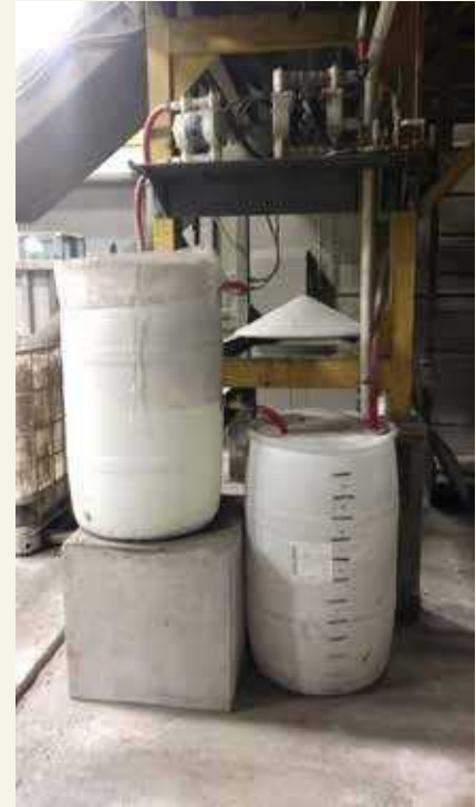
PRODUCER PLANT WINNER: Shea Concrete Products' triple filtering system for process water
