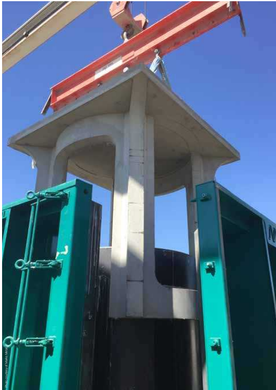
Above: Marks Metal manufactured a custom form for Pre-con's new stormwater detention product.
