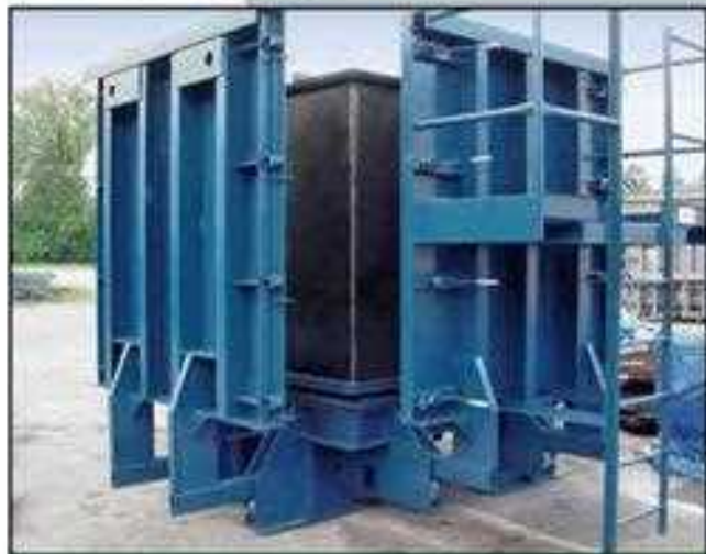
CATCH BASIN WITH ROLL BACK JACKETS
