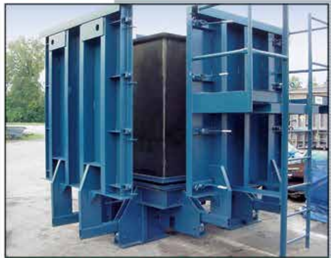
CATCH BASIN WITH ROLL BACK JACKETS
