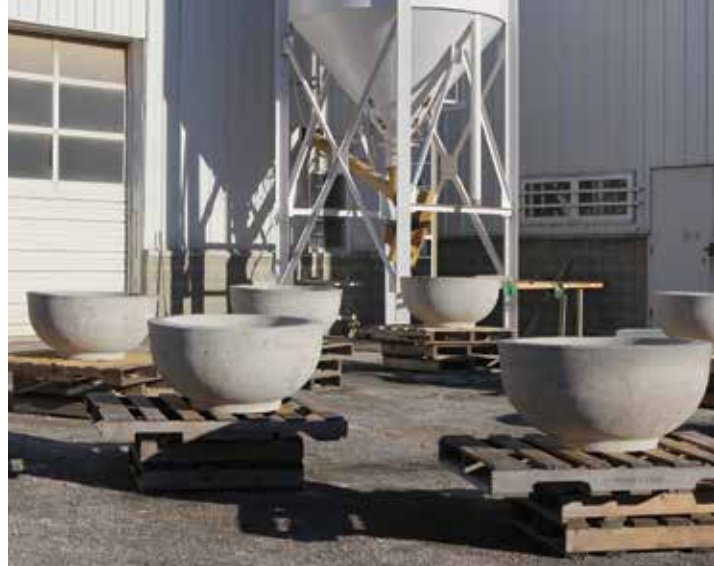
PRECAST PLANTERS AWAIT A CONTRACTOR FOR SANDBLASTING.
