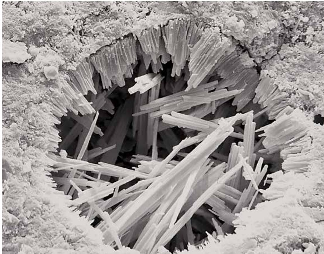
For example, the Seabrook Station Nuclear Power Plant in Seabrook, N.H., opened in 1990. By 2012, ASR was observed in some of the concrete at the plant. Testing revealed the concrete lost 22% of its original strength.<sup>1</sup> Thankfully, steps have been taken to combat the ASR at Seabrook, but how can we prevent it from occurring in the first place?
