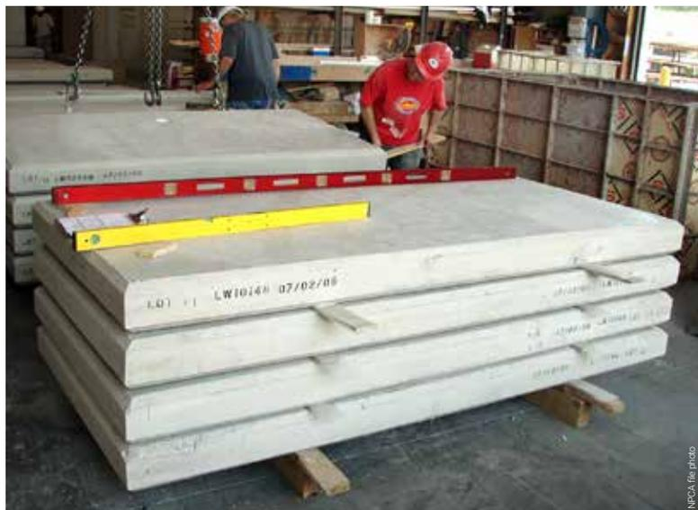
Precast products stacked with dunnage allows workers to easily slip lifting rings around them for moving in the yard and transportation.
