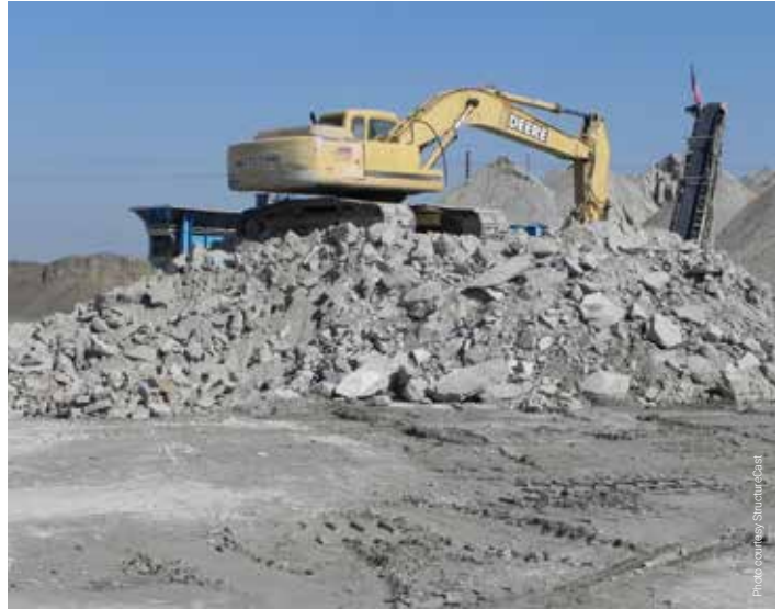
The crushing and screening plant StructureCast set up was created primarily to recycle the remnant concrete and washout material from three area businesses.
