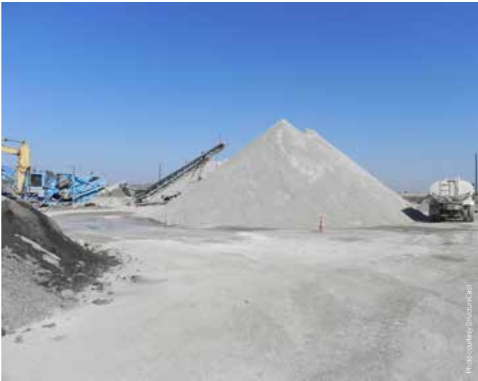
The crushing and screening plant StructureCast set up was created primarily to recycle the remnant concrete and washout material from three area businesses.
