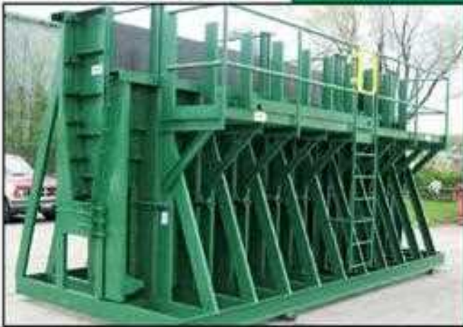
ASYMMETRICAL MEDIAN BARRIER FORM
