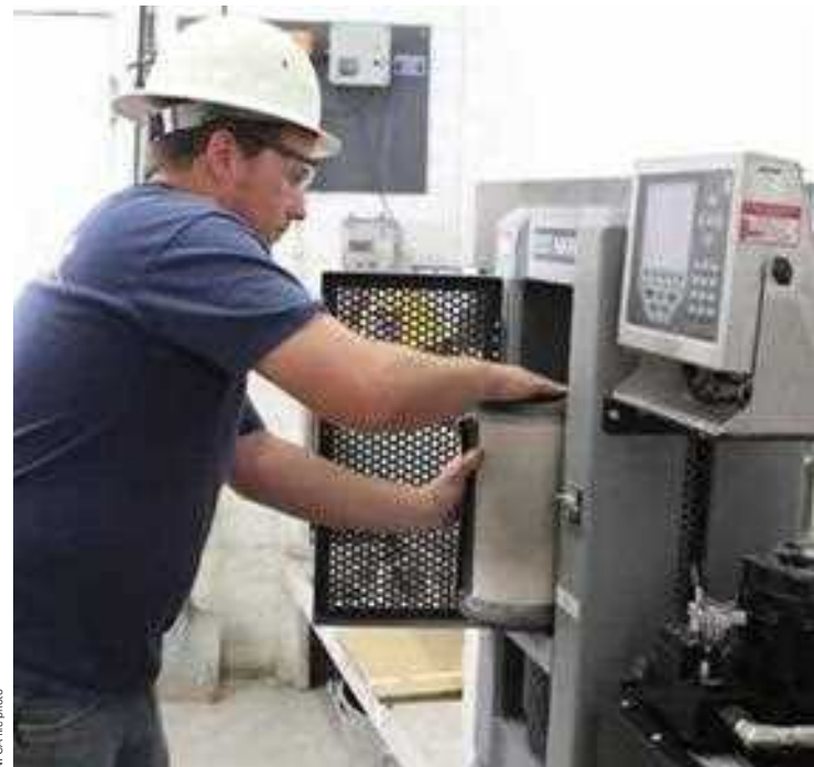
MATT ANDERSON PLACES A CONCRETE CYLINDER INTO THE STRENGTH TEST MACHINE IN THE COMPANY LAB AT PRO-CAST PRODUCTS IN HIGHLAND, CALIFORNIA.
