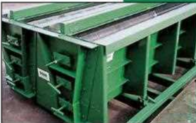
DUAL-CAVITY MEDIAN BARRIER FORM
