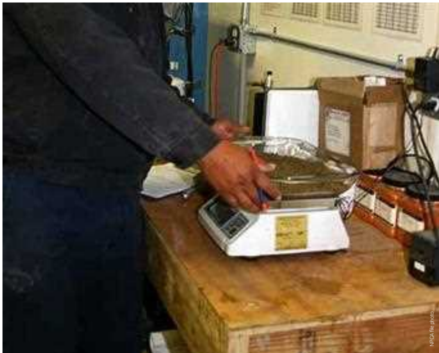
The NPCA QC Manual requires plants to determine the moisture content of each aggregate at least once daily in accordance with ASTM C566 or ASTM C70.
