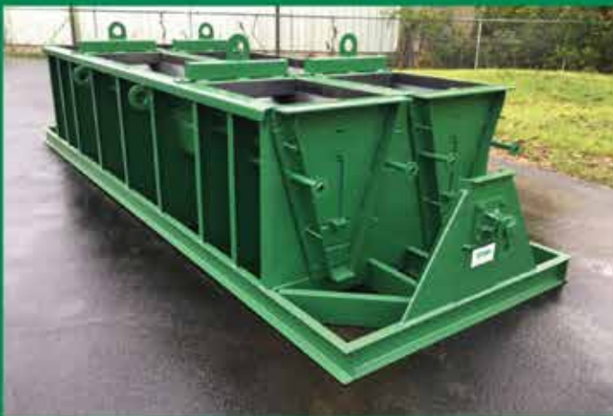
Dual Cavity Median Barrier
