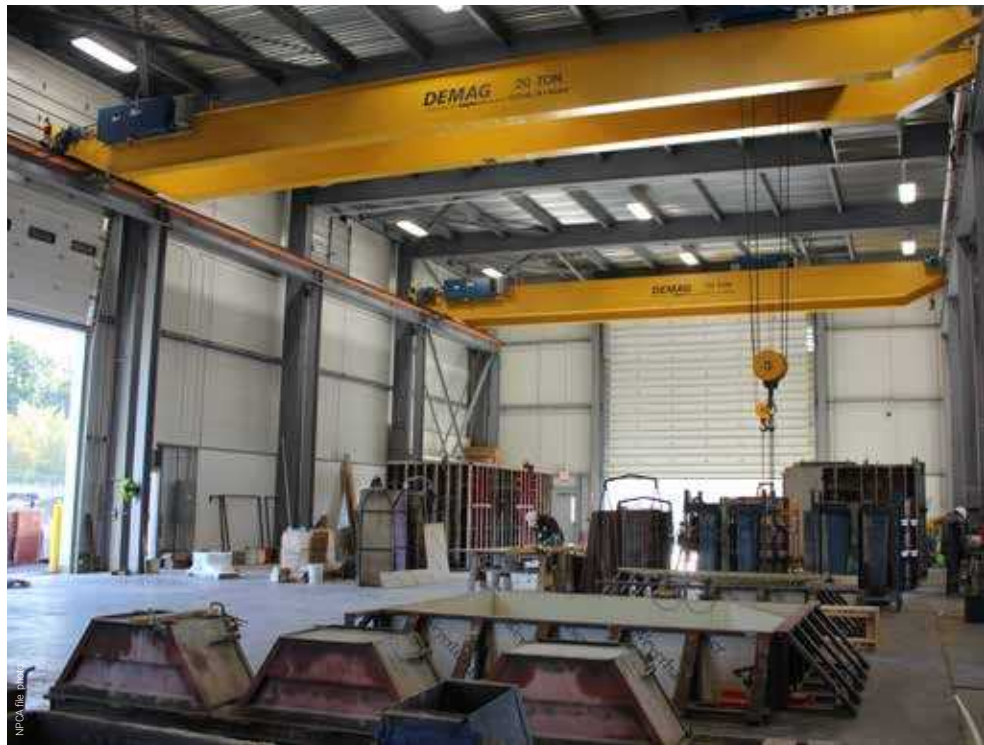
The two 20-ton bridge cranes in the new facility (below) offer the company the ability to produce larger precast products indoors. The old facility (left) still stands next door.
