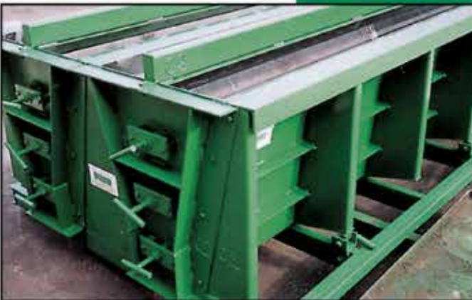
DUAL-CAVITY MEDIAN BARRIER FORM
