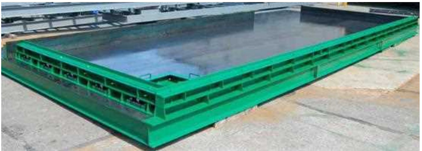
NEW FORM WORK AT ROMAN STONE CONSTRUCTION CO.
